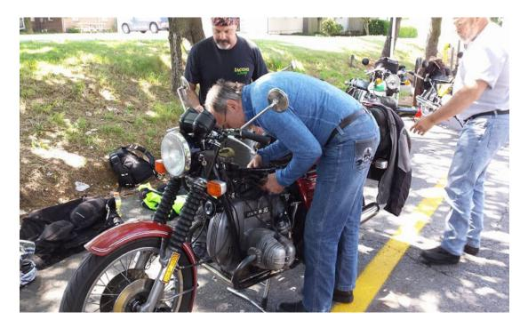
I knew very little about Joel going into this escapade but quickly determined while watching him that he was no ordinary weekend mechanic. He very methodically went through diagnosing the ignition system, ultimately determining that part of an electronic ignition conversion the bike had received was the culprit. Naturally of all the spare parts carried on the BMW the offending piece was not one of them. The BMW was effectively dead.
