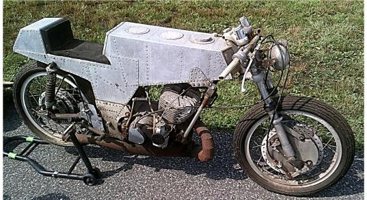
Above: an incredible barn-find displayed in the pits: a Kawasaki Bighorn monocoque framed road racer from the 70's. This one-off ultra-lightweight rotary valve two stroke was quite competitive and technologically advanced with its handmade, riveted aluminum monocoque chassis which incorporated the fuel tank. I hope it gets restored and raced again. *Simply awesome!*
