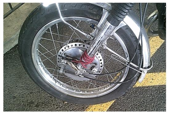
On Monday morning we again pass through Berkeley Springs, then take Route 522 north, crossing the narrowest part of Maryland before popping back into Pennsylvania. The Suzuki's drum front brake has begun to stick. We make a quick temporary repair after liberating a bungee
