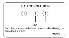
To reverse direction of rotation interchange connections L1 and L2.
