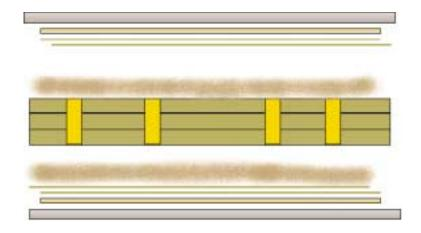
Steel Caul Plate Copper Foil or Release Film Prepreg Backer
